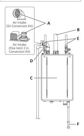
[When supplying combustion air from the indoors] For smear or blockage with dust, oil, etc. at the air supply vent.
