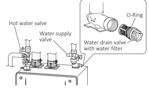
2. With a bucket ready, remove the water drain valve.
