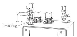
8. When the water is completely drained, reattach all drain plugs and close the hot water fixtures/faucets.
